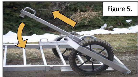
If needed, the spring-loaded pin can be adjusted, to ensure that this pin fully snaps into place. To do this, first loosen the round black knob and inside nut next to the knob. This will allow more of the pin to extend into the cart frame. Once the spring-loaded pin is set to the desired length, tighten the black knob and nut together to lock this adjustment in place.
